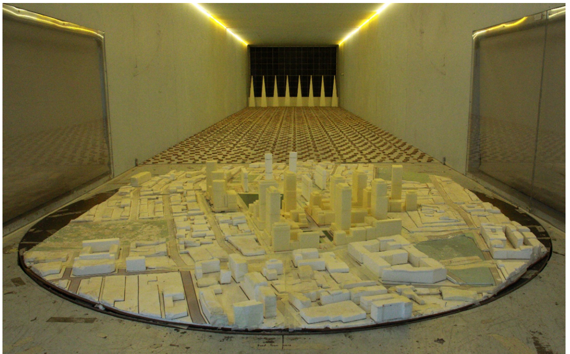
Figure 9c: Photograph of the Wind Tunnel Model – (View from the South)
